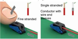
5. To loosen a conductor, always push finger-operated levers.
