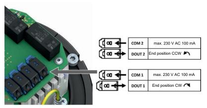
Figure 9: Plug-in terminals option 2, multi I/O module
