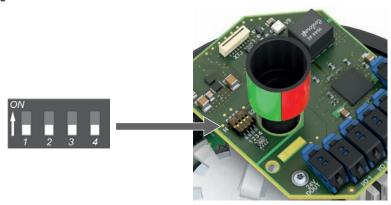
The inputs and outputs of the multi I/O module can be configured using a DIP switch.
